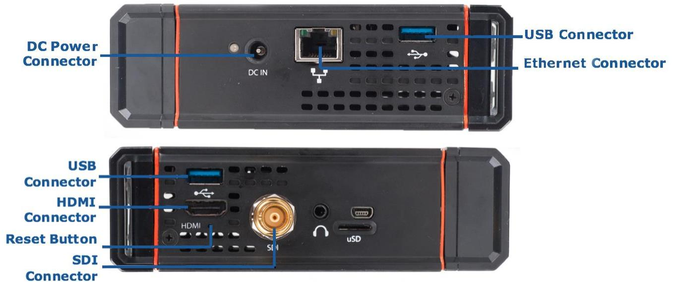
The procedure for connecting a video camera to the LiveU Solo is simple.
